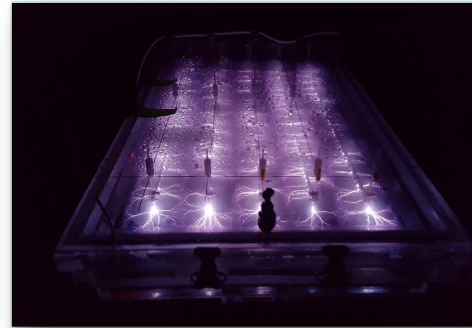
Pilot-scale plasma reactor for IDW treatment (Singh et al, ES&T, 2019)
